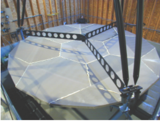
Figure 6.3. The 6-meter LZT primary mirror under construction (P. Hickson).
