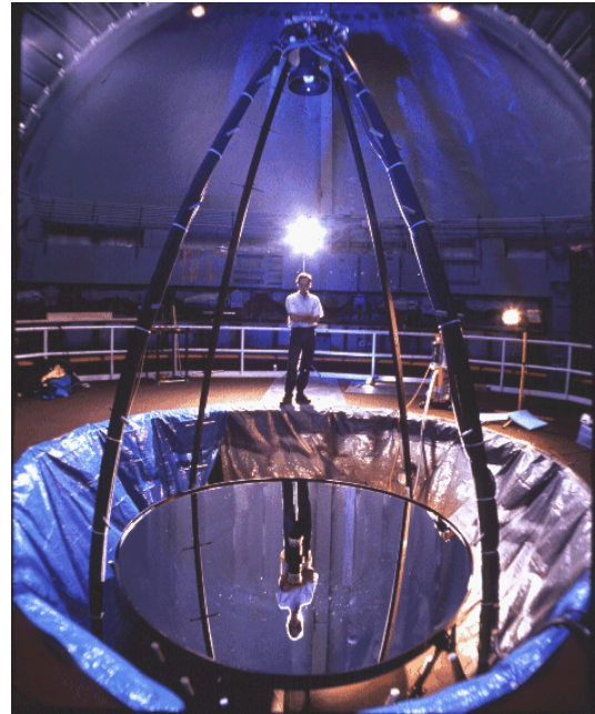
Figure 6.1 The 3-meter liquid-mirror telescope of the NASA Orbital Debris Observatory (C. Simons).
