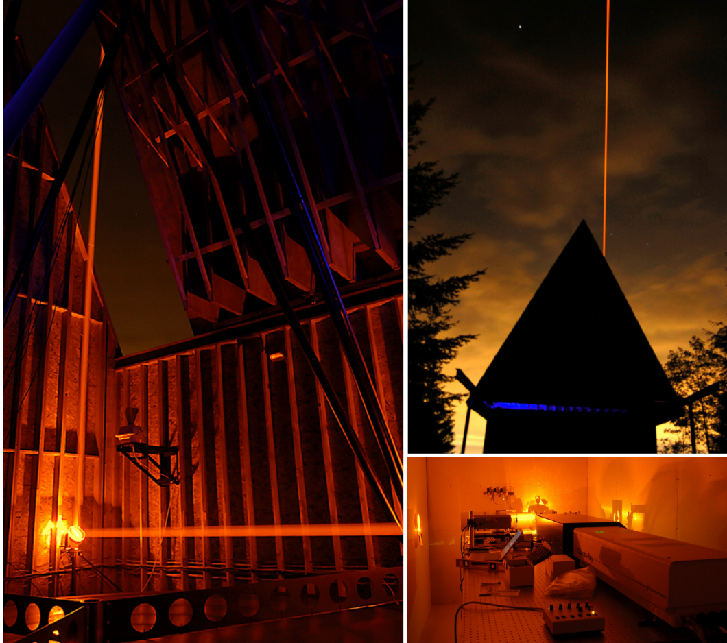
Figure 4. First light of the laser launch facility. On the left hand site, parts of the stabilizing spider of the 6-m mirror, the hexapods of the prime focus, the 25 cm flat and the safety radar as well as the lidar beam are visible. On the right hand at the bottom, the laser room in action is shown and the LZT enclosure with the uplink beam and a partly opened roof is visible in the upper part. The blue light is caused by the laser warning LEDs.
