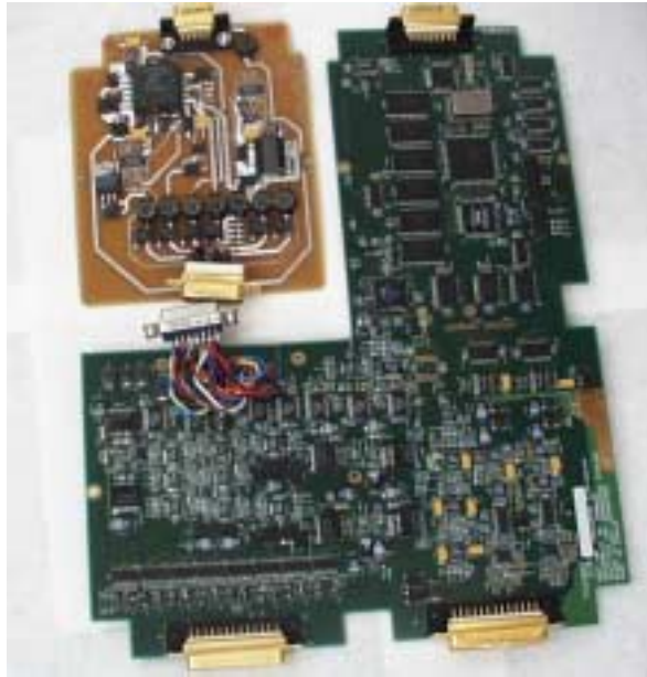
Figure 7: Instrument Computer (power supply shown in upper left)
