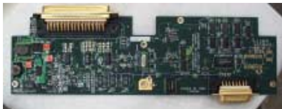
Figure 10: Telemetry and Command Node – modem and telemetry collection
