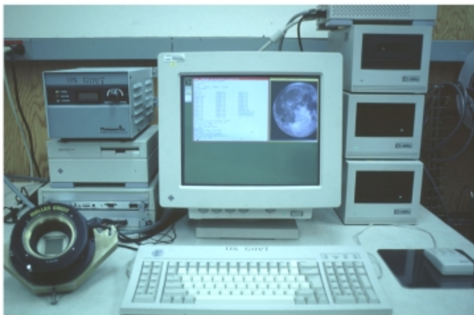
Figure I-5. View of the Lick-Smithsonian-Photometrics (LSP) 2K CCD and support equipment used with the NASA-LMT during the 1994 through 1997 observing seasons. This 15 micron pixel 2048x2048 array CCD yielded a 20.33 arcminute wide field of view. The computer system has since been upgraded and the LSP 2K CCD has been replaced with 1K and 2K CCDs with higher quantum efficiency.
