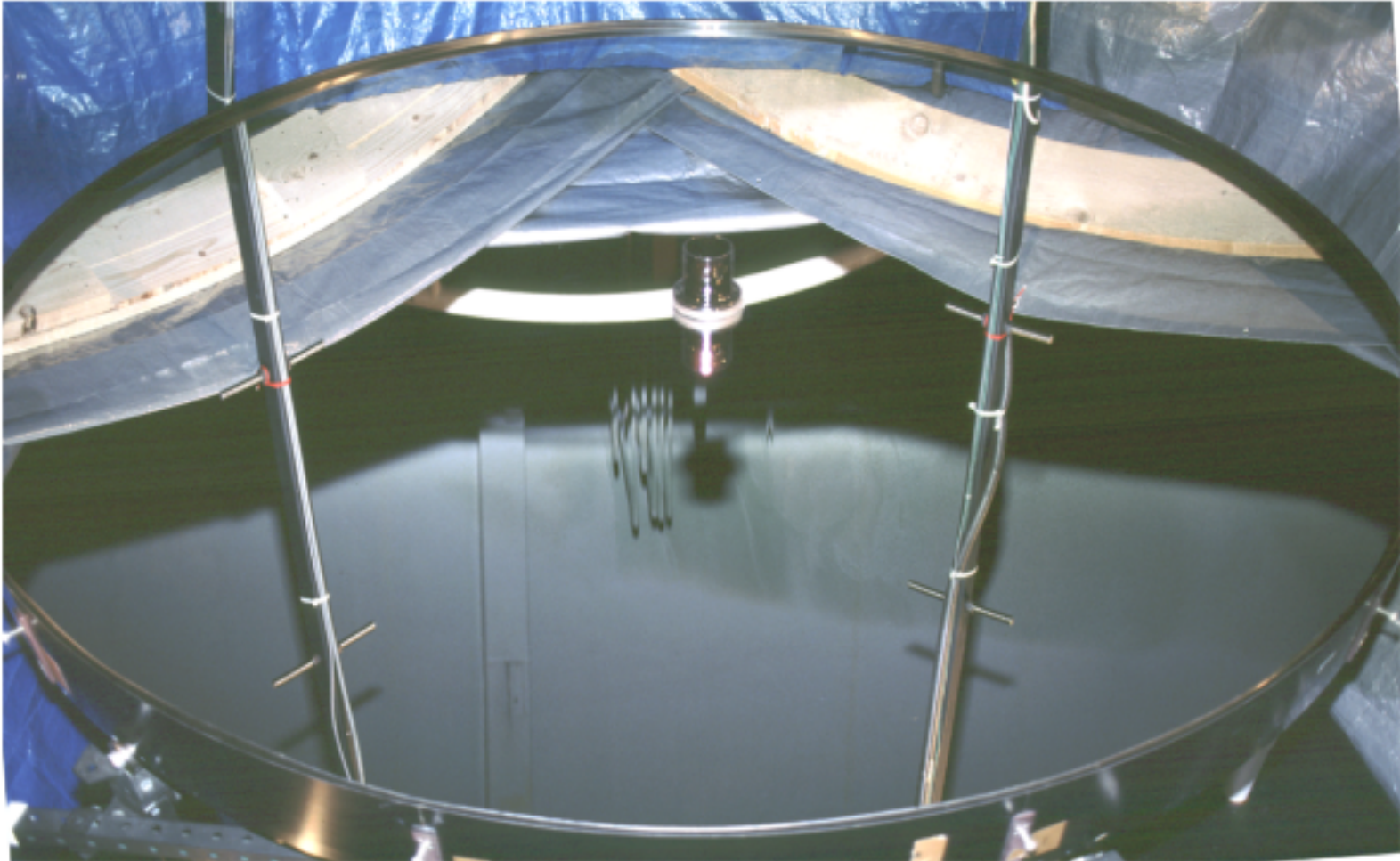
Figure I-2. Close-up of the 3.0 m diameter NASA Liquid Mirror. The mirror is spinning at an angular velocity ( \omega ) of 1.043107 radians/second yielding a parabolic surface with a 4.511 m focal length ( f/1.503 ) at the NODO location ( g=9.8167 \text{ m/s}^2 ).
