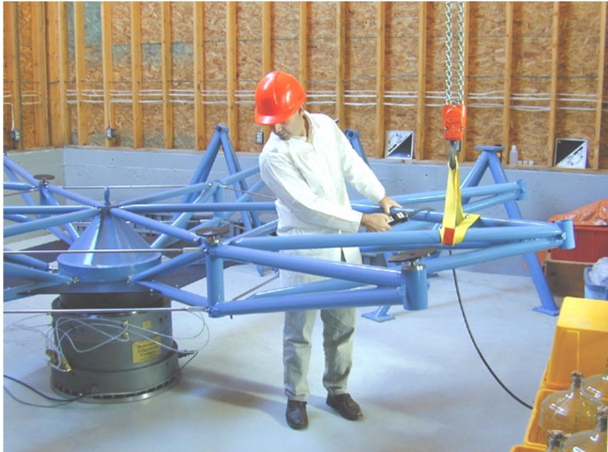
Figure I-17. Assembling the space frame for the 6.0 meter diameter Large Zenith Telescope (LZT). Several floatation pads which will support the mirror membrane are visible. The PICO 20R air bearing is seen with the plexiglass protective cover not yet installed. Photo courtesy Paul Hickson.
