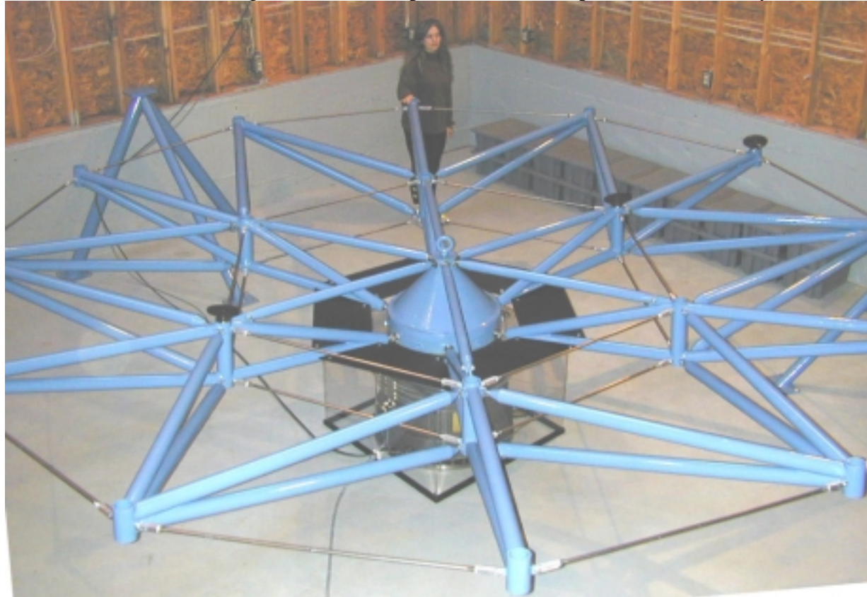
Figure I-16. The 6.0 meter diameter Large Zenith Telescope (LZT) designed and built by Paul Hickson at the University of British Columbia (UBC). The space frame design of the mirror substructure is an alternative to the monolithic composite construction presently employed in LMT primary mirrors. A thin composite membrane will be placed atop the space-frame and will be supported by floatation pads that can be adjusted to give an overall parabolic figure to within a \pm 0.1 mm surface deviation. The final mirror will support a 1mm (or thinner) Hg layer and operate at f/2 . The Professional Instruments Company (PICO) air bearing, which was specially designed for this project, is enclosed in a plexiglass cover beneath the structure. It can support a 9,000 kg axial load - sufficient for an 8 meter LMT. Photo courtesy Paul Hickson.
