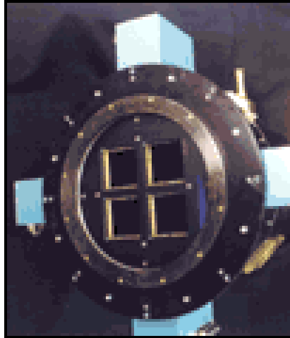
Figure 2.23 The Big Throughput Camera (BTC) – a mosaic of four 2048×2048 pixel CCDs. The CCDs are housed in a vacuum dewar and cooled with liquid-nitrogen to approximately 170 K.
