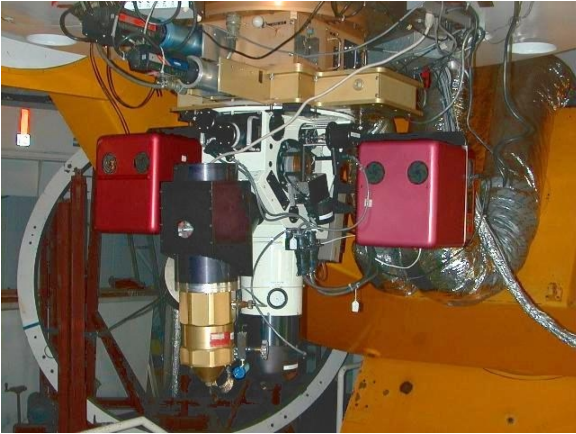
Figure 5.1 The Boller and Chivens CCD Spectrograph (the white structure) used on the MDM Observatory 2.4-m and 1.3-m telescopes. It is a conventional optical grating spectrograph operating in the 3200 - 9500 Å region. Seven gratings are available providing spectral resolutions between 550 and 9100. The slit width is continuously adjustable between 0.5 and 13 arcsec. The detector is a Loral 1200 × 800 pixel CCD (the gold coloured cylinder). Lamps mounted above the spectrograph are used for wavelength calibration and flat fielding. At the lowest dispersion, the peak total system quantum efficiency is about 19% at 5200 Å. An intensified camera records the image provided by the telescope on the polished entrance slit jaws and for an integration time of a few seconds, point sources with magnitudes just below the POSS limit can be seen over most of the 5 arcmin field of view at the 2.4-m telescope. Low resolution spectra of objects as faint as 20.5 mag can be obtained at the 2.4-m telescope.
