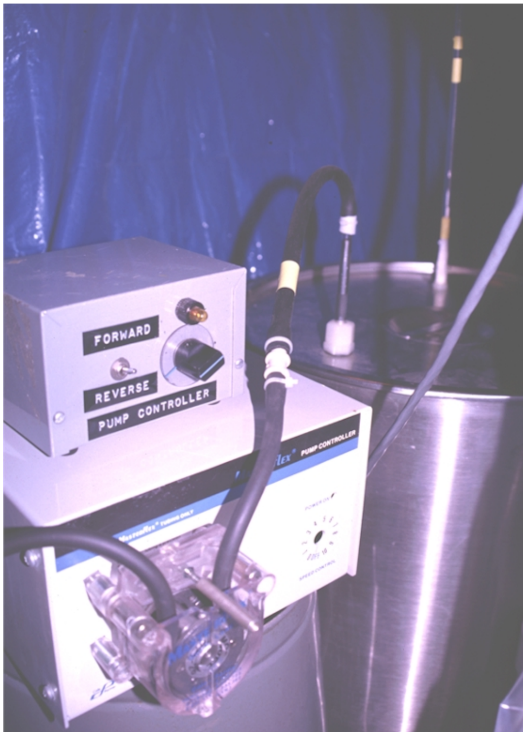
Figure IV.H-3. The Stainless Steel Hg Reservoir and peristaltic pump used for adding and removing Hg from the liquid mirror. Mercury is moved through the Neoprene tubing via peristalsis thereby eliminating Hg contamination of a pumping mechanism. A calibrated float level in the reservoir indicates the volume of Hg removed or returned.
