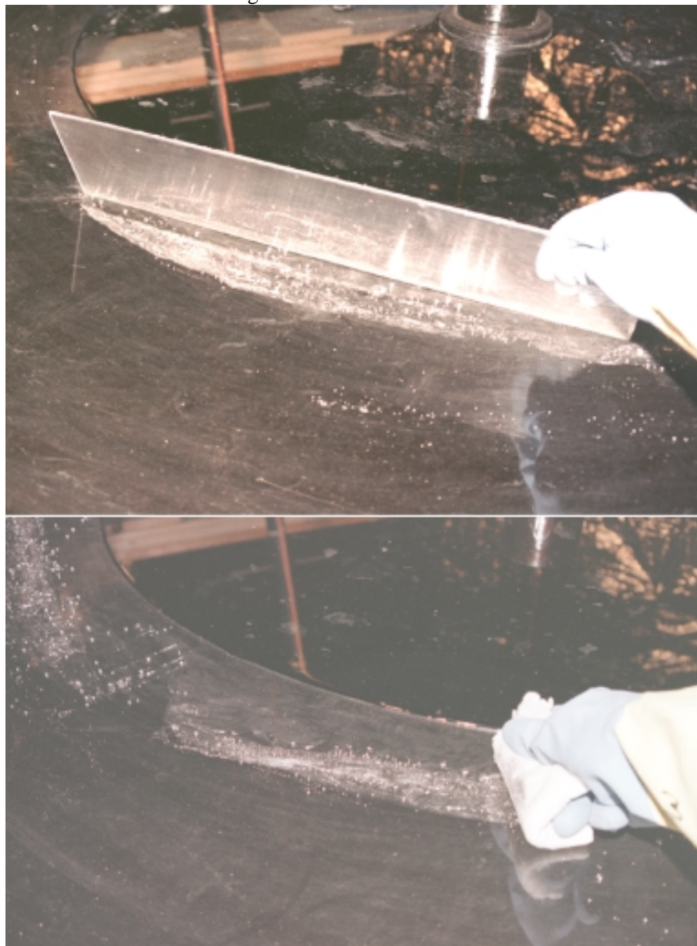
Figure V.A-6. After consolidating the material collected from each skimming pass, a surgical cotton pad soaked with Isopropyl alcohol is used to wipe clear the accumulation. The pad attracts dirt and debris, but has minimal affinity for Hg, thus limiting Hg loss during each mirror cleaning to less than 1 milliliter. Approximately 15 passes with the skimmer are required to clean the mirror and the entire process takes 1 to 2 hours depending on the amount of accumulated dirt and debris.
