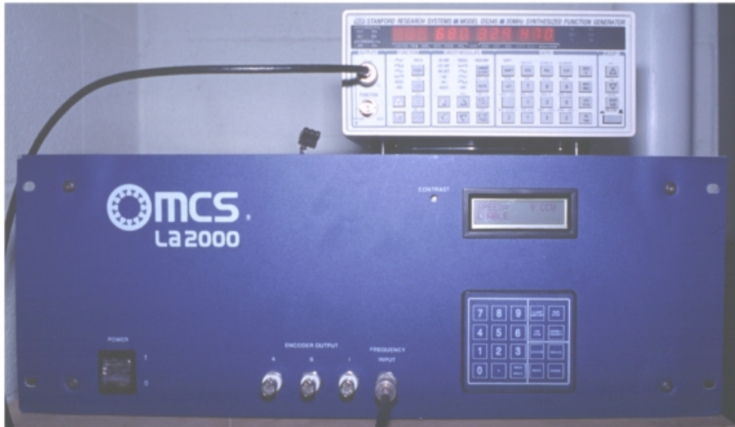
Figure IV.G-3. A view of Motion Control Systems (MCS) LA2000 3-phase sinusoidal linear amplifier with the Stanford Research Systems (SRS) function generator and 0.01 ppm time base. In the normal open-loop configuration, the function generator provides a fixed reference signal from which the linear amplifier generates a 3-phase sinusoidal output to drive the MFM 12-pole brushless DC motor that is directly coupled to the PICO air bearing .
