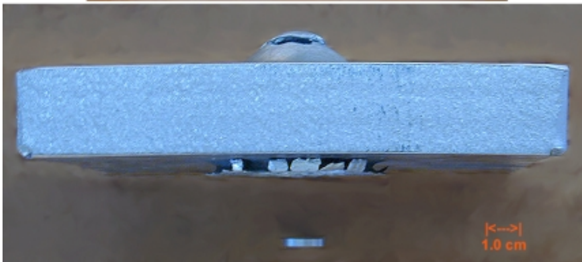
Figure II.A-1. The impact crater on a stationary 2.5 cm thick aluminum plate resulting from a collision with a 1.5 gram, 1.6 cm diameter aluminum disk, traveling at 1.5 km/sec. The kinetic energy of the disk was 1688 Joules, significantly less than the 50,000 Joule kinetic energy typical of an identical particle involved in an orbital collision.
