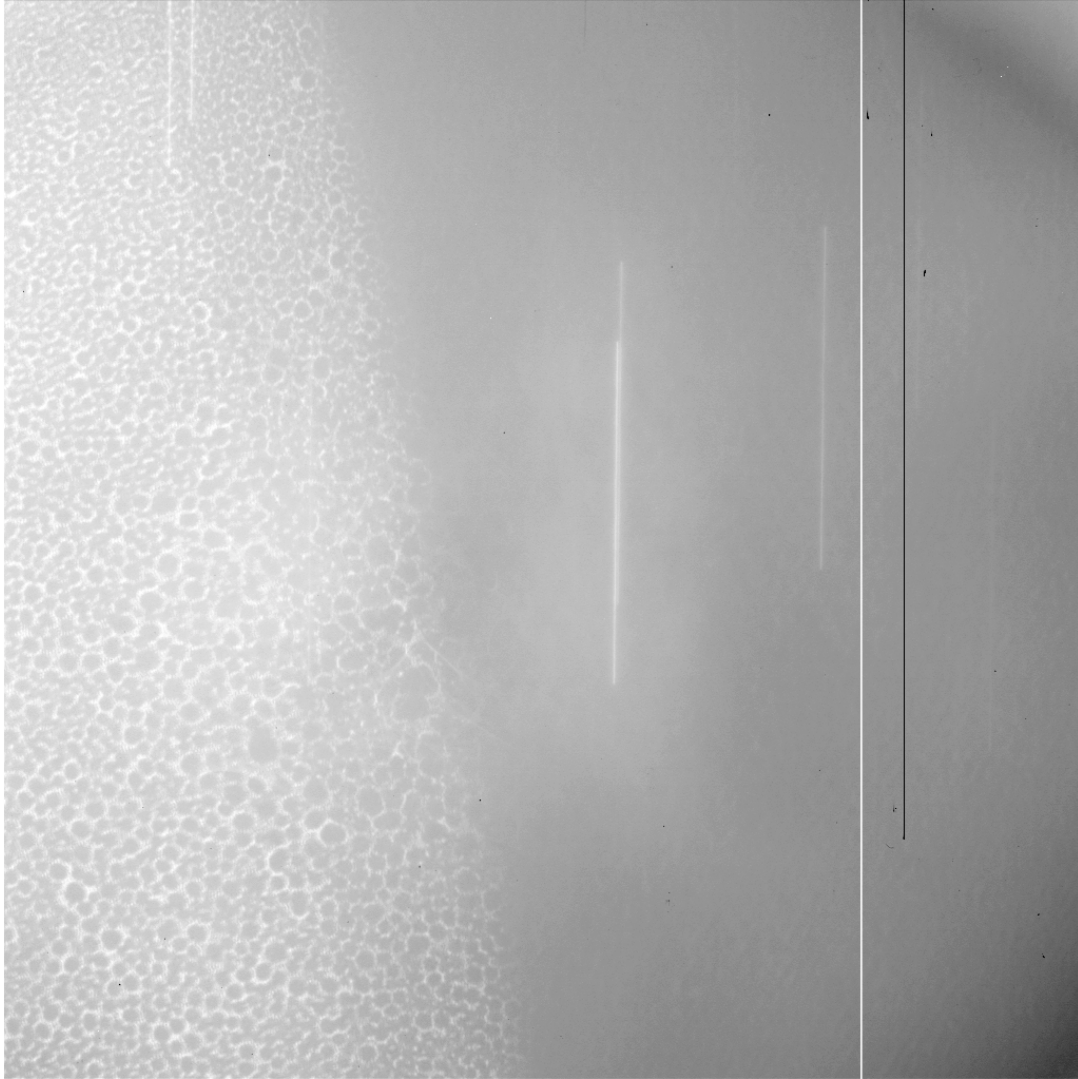
Figure V.I-2. A demonstration of the effect on image quality of moisture condensation on the CCD Camera Head optical window. Radiative cooling of the window by the CCD can cause the formation of condensate on the window during conditions of high relative humidity. The refrigerated circulating fluid which cools the Petier Thermoelectric device via a water-jacket can also cool the entire camera head below the dew point. This can result in the formation of a tremendous amount of condensation as in this example. The shadow of the water droplets are clearly visible on the left side of the field on this moonlit night at NASA-JSC. Only rarely does dewing this severe occur at NODO. As with the condensation induced from radiative cooling, the introduction of a clean dry air stream ( -30^{\circ}\text{C} dew point) across the CCD window helps mitigate this problem as long as moisture does not migrate into the field from the body of the camera head. Image was acquired with the LSP 2K CCD.
