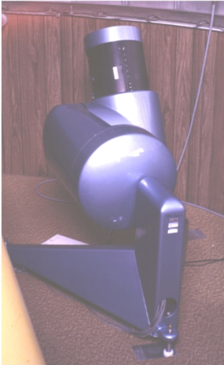
Figure II.A-4. Photograph of the NASA-CCD Debris Telescope (NASA-CDT). This 32 cm diameter Schmidt camera has a three-axis mounting developed by Jim Wray enabling it to track orbiting objects . It is presently installed at NODO where it primarily searches for orbital debris at GEO altitudes.
