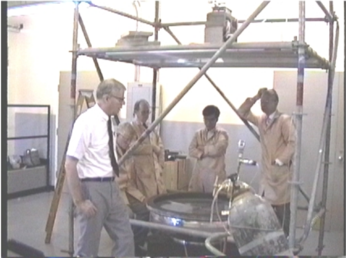
Figure IIB-10. View inside JSC building 268 showing the prototype 1.0 meter diameter LMT. This image was acquired after a spin-casting trial with epoxy in which excess air entrapment occurred. The scaffold enabled access to the mirror's radius of curvature for Foucault testing of the mirror's figure. The nitrogen bottle in the foreground provided backup in the event of an air system failure. NASA Branch Chief Drew Potter, the initiator of the project, is at left.
