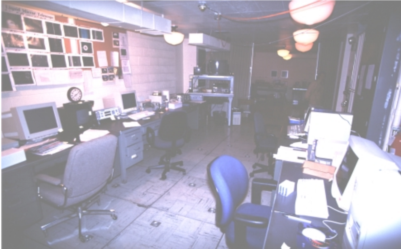
Figure II.C-9. The control room at NODO. The majority of LMT operations are controlled from this room located on the second floor of the NODO facility. Telescope control lines run 40 m from the dome level two stories above. Only the motor controller and the Digital Video (DV) recorder for the orbital object camera are located near the telescope since they require short cable lengths. All equipment is tied to Uninterruptable Power Supplies (UPSs) and an Emergency Generator. Unix machines (left) control the CCD camera, WinTel PCs (right) provide data logging and storage, the Intensified Video camera for orbital object data acquisition is controlled from the station at the rear. All machines are networked with Internet access.
