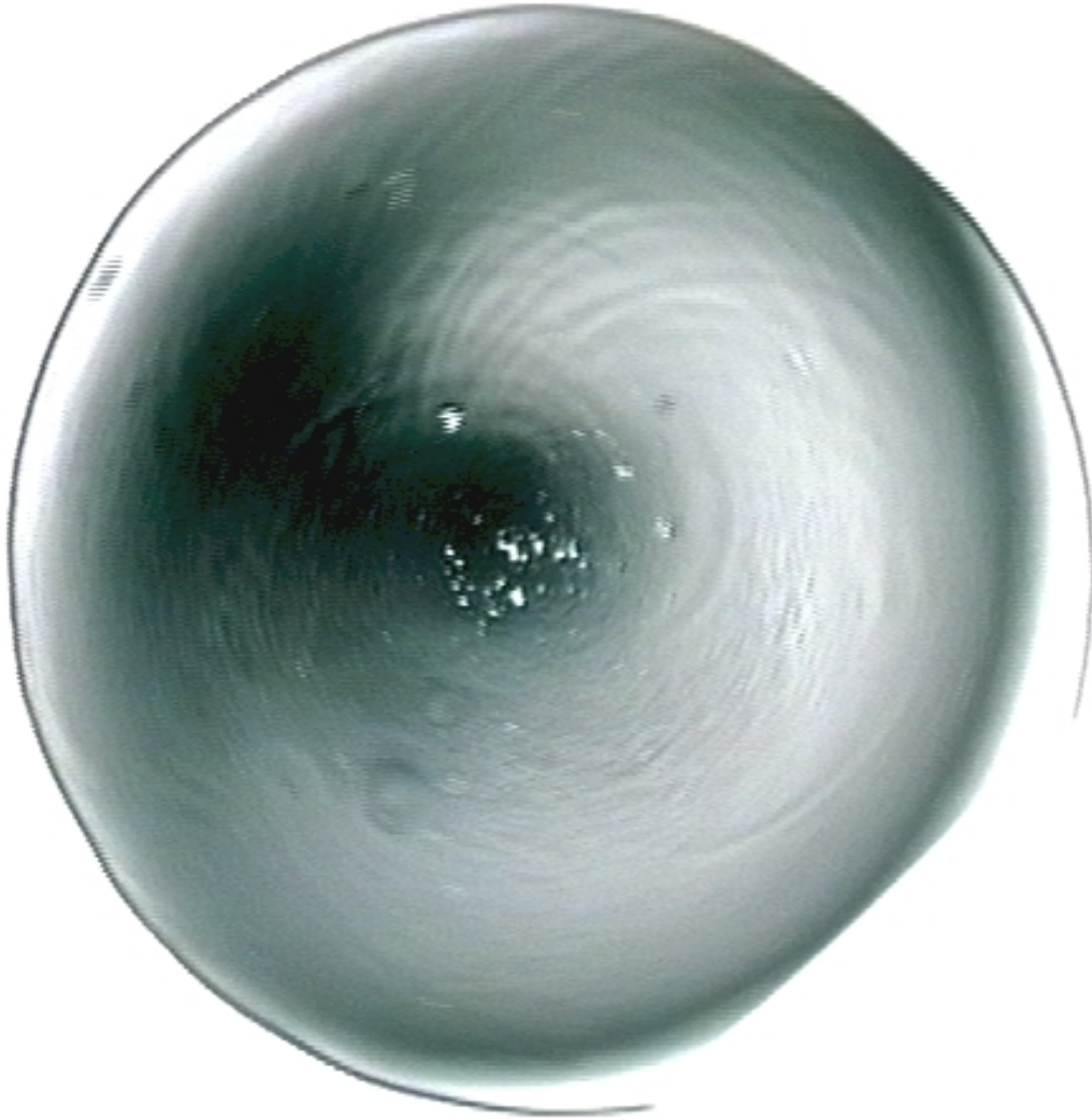
Figure II.B-12. View under point source illumination and knife-edge of the prototype 1.0 meter diameter LMT using liquid water as a reflective medium. This is the same image as in Figure II.B-11 except inverted to show the continuation of the spiral wave pattern.
