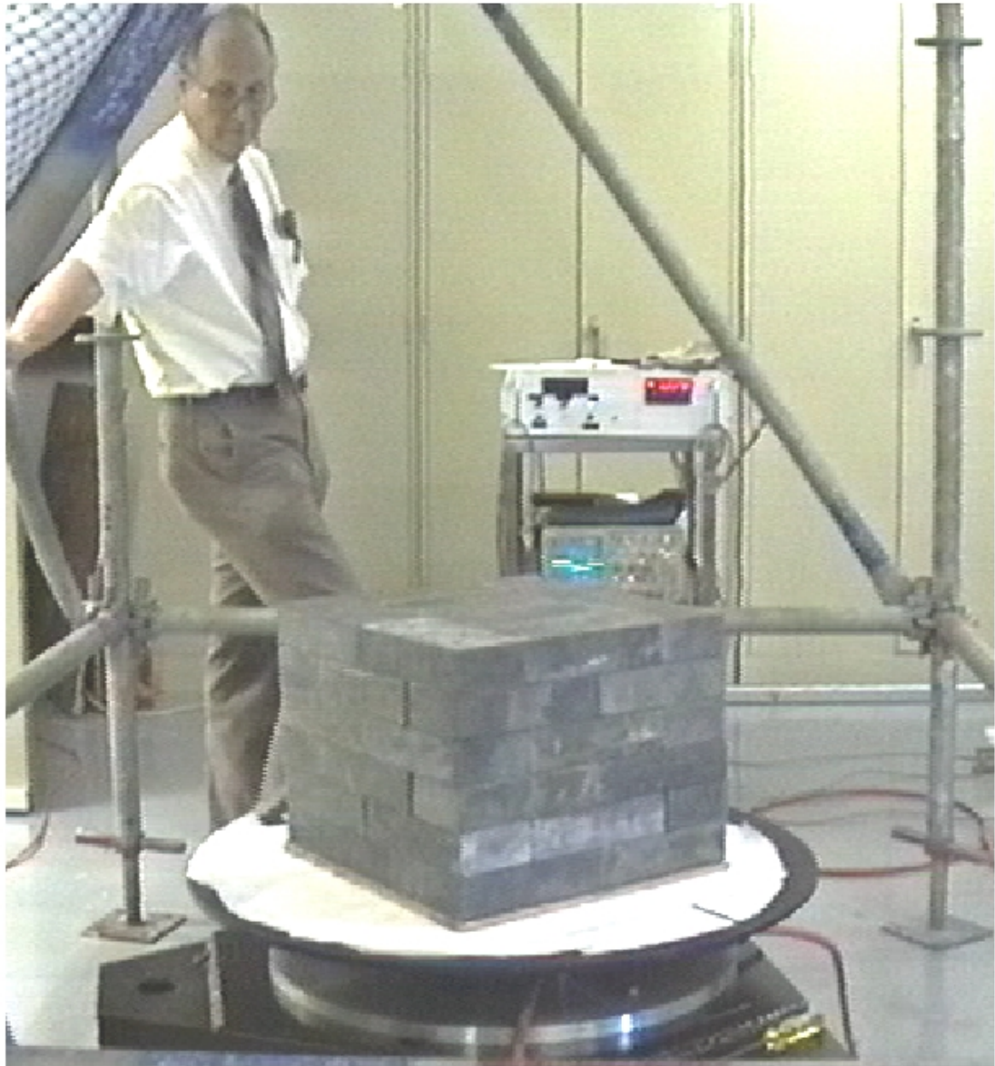
Figure II.B-8. View inside NASA-JSC building 268 showing the prototype air bearing involved in an axial load test. The Warren air bearing has been axially loaded with 545 kg of lead bricks, thus duplicating the anticipated load of the 3.0 m mirror (160 kg) and a maximum 4 mm thick layer of Hg (390 kg). A suitable air bearing must satisfy both axial and angular load capacity criteria, but in this test, the bearing could not sustain the load without binding during rotation. Modifications were later made which enabled the bearing to successfully support a 680 kg load. The bearing was also able to meet the angular load capacity criteria (Chapter IV), but ultimately failed due to an oscillatory instability. The bearing was replaced with the completely successful PICO air bearing. Engineer Frank Gibbons, the original Lockheed Project Manager, is in the background with the drive electronics at his left.
