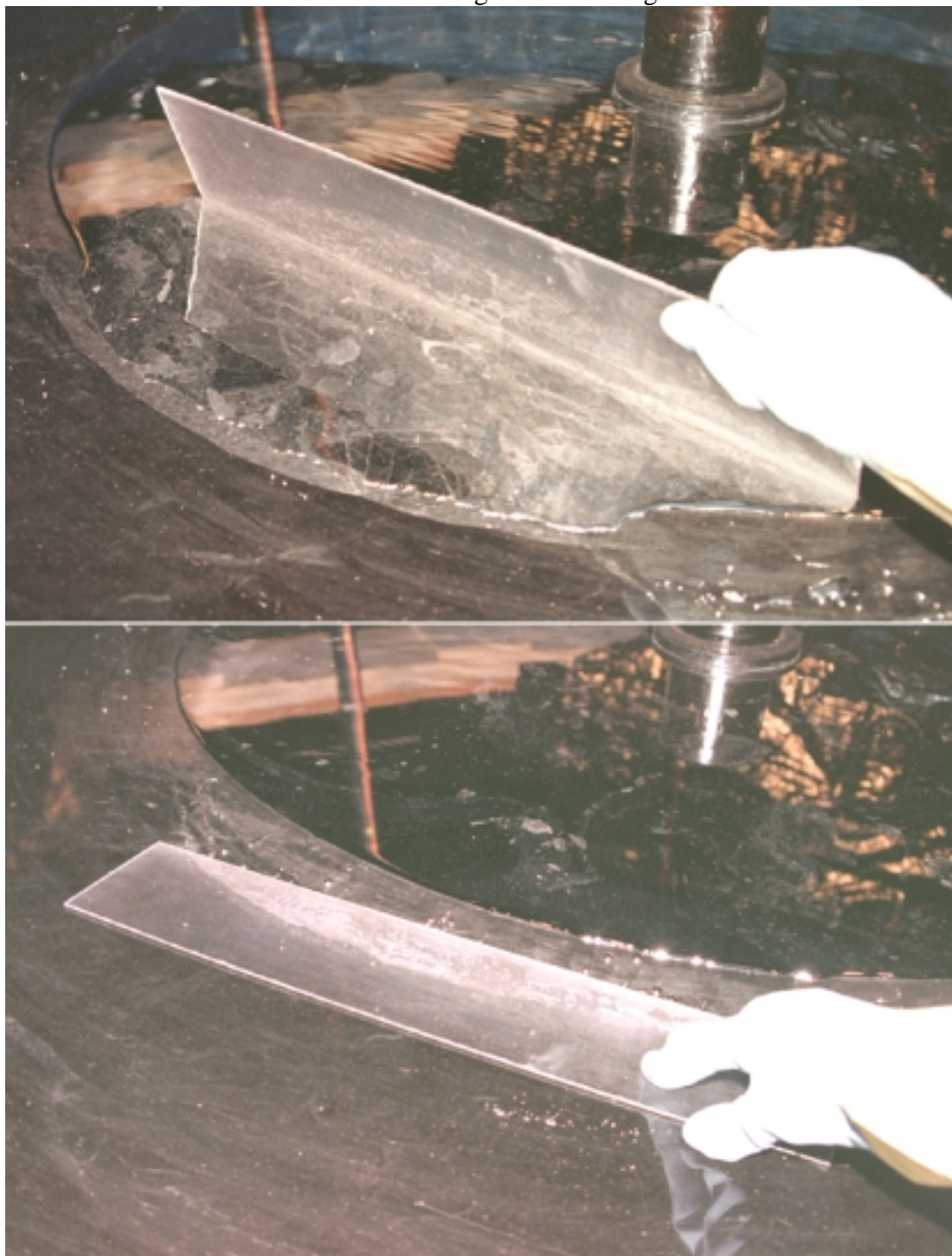
Figure V.A-5. The central Hg pool is cleared of dust, debris, and oxide by using a plexiglass or LEXAN skimming tool. The tool is used to drag elements of the surface film to the mirror substrate adjacent to the pool. The tool is then laid flat against the substrate to consolidate the collected material.
