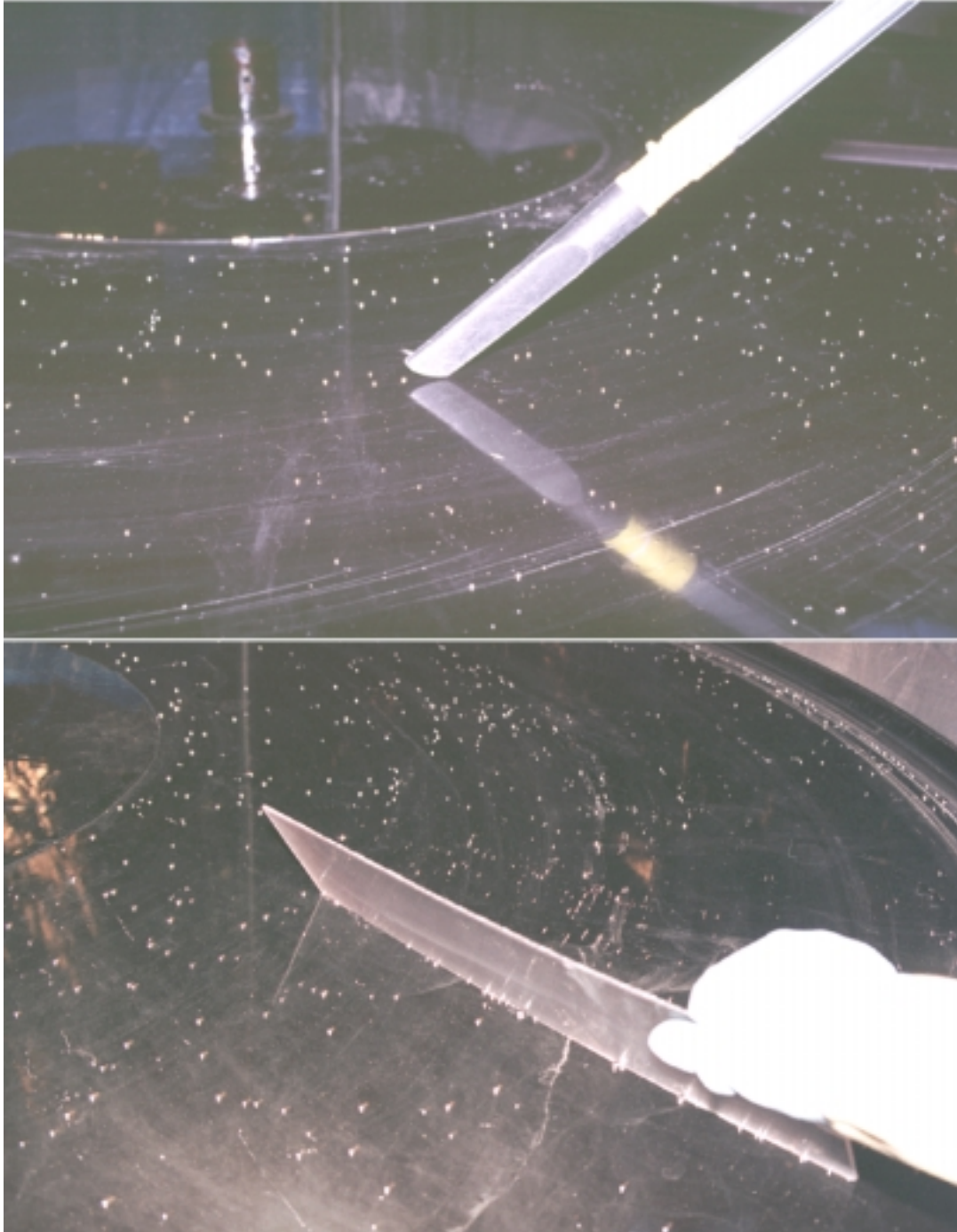
Figure V.A-4. After the perimeter channel is drained, large pieces of debris are removed from the polyurethane mirror substrate using the Hg vacuum cleaner (upper photo). (The vacuum is also used during mirror formation to extract stray pieces of debris at the sites of Hg surface tears.) Once large debris is removed, the skimming tool is used to clear the mirror substrate of all residual Hg droplets. This helps eliminate the loss of Hg when the substrate is wiped clean at the conclusion of the cleaning process.
