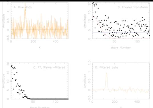
The raw data of A is a Gaussian sitting on a flat baseline, with random Gaussian noise added. The DFT in B shows the signal and noise components, modelled by the Gaussian and horizontal curves respectively. The Wiener filter, applied in the frequency domain, produces the DFT of C, and the reverse transform produces the greatly improved s/n of D.
