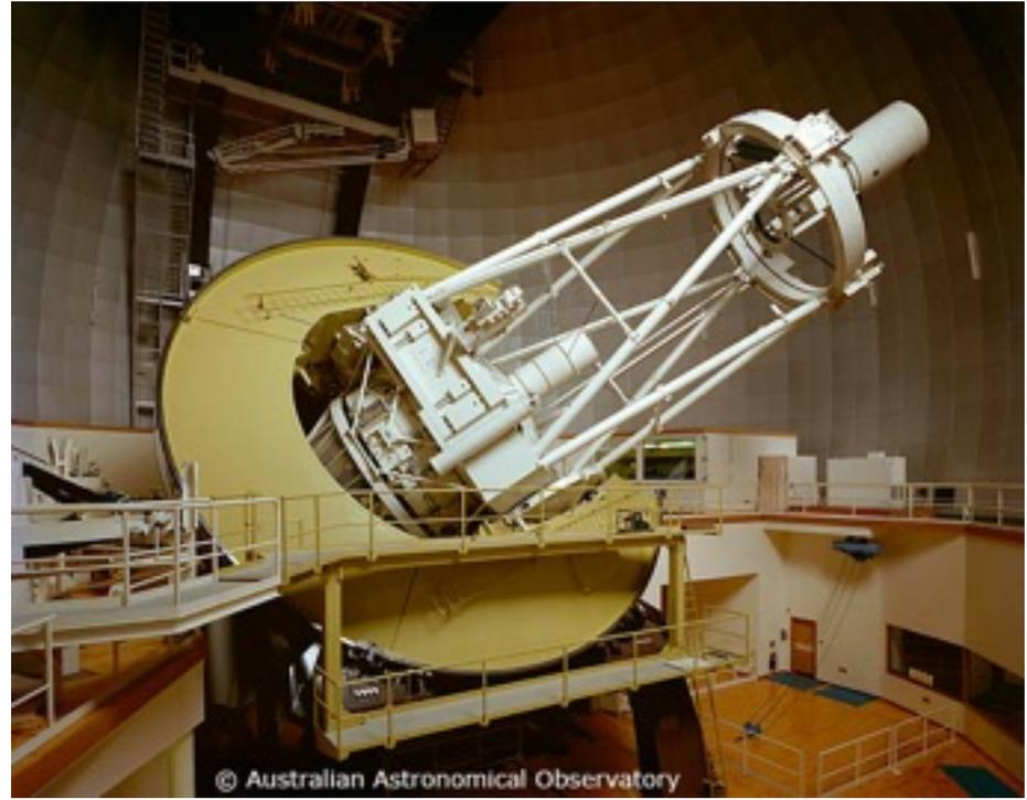
The Anglo-Australian Telescope: 3.9 m equatorial mount (the last!) at Siding Spring Observatory, Coonabarabran, NSW, Oz
